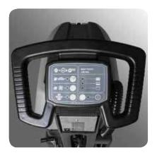
On/off switch protecting unintentional use. Protection against overloads, battery discharge abuse (DC only) and undesired run. Convenient one switch maintenance over the brush. Eco Energy setting for extensive working time and extremely quite operations (DC only).
