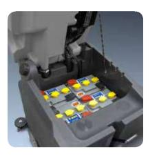
Great working autonomy thanks to the possibility to use 4 batteries 6 V 180 Ah granting continuous working up. Possibility to use also 2 batteries 12V. Less battery consumption thanks to rear wheeldrive. Large load tanks made of shock and acid proof polyethylene (real load of 85 l.), avoiding frequent stop for refilling.
