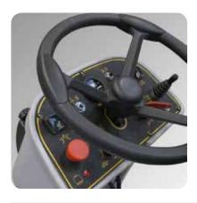
Comfort M scrubbers are easy to use thanks to the simple and user friendly controls. From the control panel the operator can adjust the maximum forward speed and the quantity of cleaning solution outflow, selecting the options most suitable to the dirt type. Job is simplified and made faster by the automatic lifting of the squeegee and of the brush plate.
